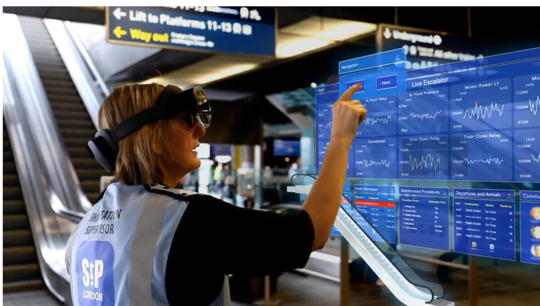
Figure 16 – An example of how live monitoring data for lifts can be explored to diagnose faults remotely
