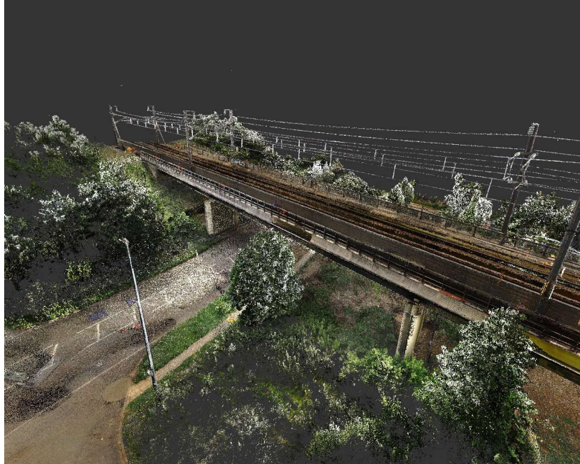
Figure 17 – 3D BIM model of HS1 bridge asset
